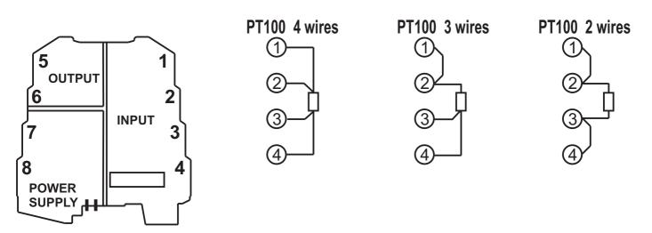
The PT100 measure is effected in impulsive way for a very short time to reduce the module consumption. For this reason, some electronic calibrators could not be able to generate the simulated signal in the right way.
