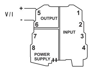
Note: in order to reduce the instrument's dissipation, we recommend either using the output for voltage or guaranteeing a load of > 250  $\Omega$  to the current output.
